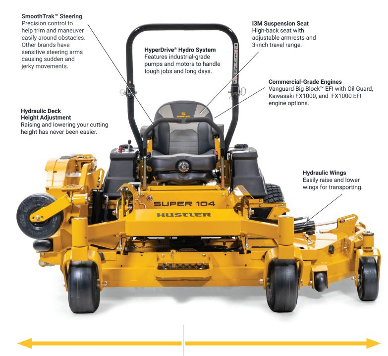
80" Transport Width Fits most trailers making it easy to transport from job-to-job. **104" Width of Cut** Widest and most productive commercial zero-turn available
