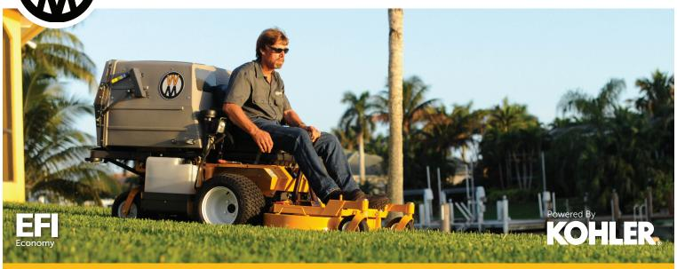
Operators can expect easy starting, consistent running temperatures, and user-friendly maintenance from this top-of-the-line mower. A combination of liquid cooling and EFI from Kohler's 30-HP Aegis engine provides increased engine life, power, and better fuel economy compared to air-cooled engines.
