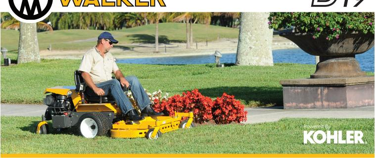
The B19 is a simple, clean design using many of the same principles as the Walker original. At the heart of the B19 is a Kohler Command engine and a simplified drive train. Decks are easily installed and changed using the quick disconnect PTO drive shaft.
